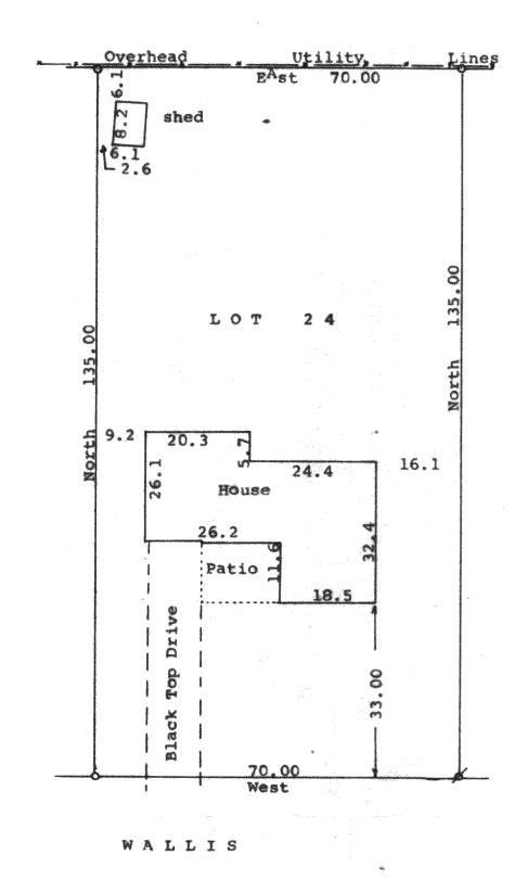
Scale - 1" = 20' o= 1" Iron Pipe Found ø= 3/4"Iron Pipe Found Bearings referenced to the recorded bearings on the Plat of Delmar Survey ordered by: Assured Realty, Inc 50 West Geneva
